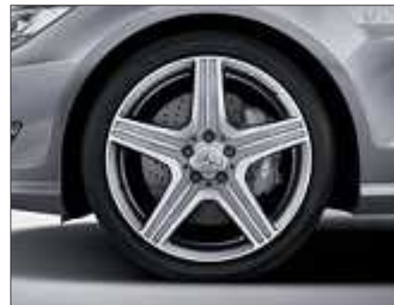
Triple-spoke AMG light-alloy wheels with 255/35 R 19 front and 285/30 R 19 rear tyres, painted in titanium grey with a high-sheen finish (standard for CLS 63 AMG, Code 797).
