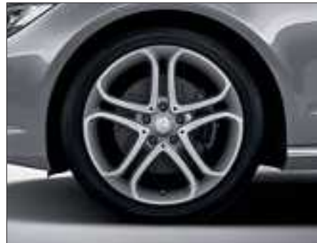
5-twin-spoke light-alloy wheels with 255/40 R 18 front and 285/35 R 18 rear tyres, bichromatic, painted in himalayas grey with a high-sheen finish (optional, Code 22R).
