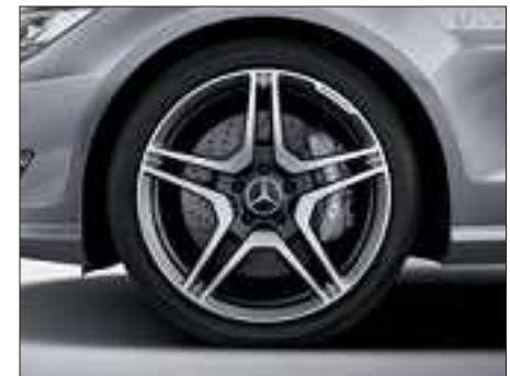
Twin-spoke AMG forged wheels with 255/35 R 19 front and 285/30 R 19 rear tyres, painted in titanium grey with a polished surface (optional for CLS 63 AMG, Code 793).
