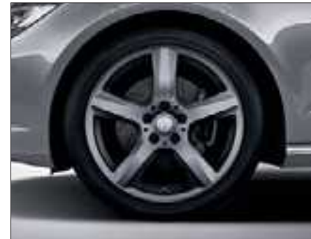
5-spoke light-alloy wheels with 255/40 R 18 front and 285/35 R 18 rear tyres, painted in silver (standard for Exterior Sports package, Code R32, in anthracite Code R36).
