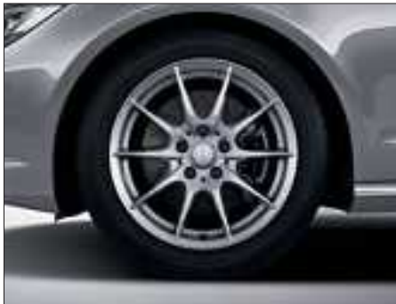
10-spoke light-alloy wheels with 245/45 R 17 tyres (standard for 6-cylinder models and CLS 250 CDI Shooting Brake, optional for CLS 250 CDI Coupé, Code R43).
