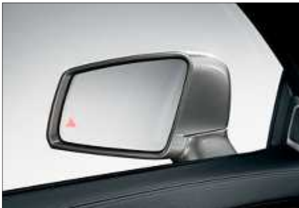
Lane Keeping Assist and Blind Spot Assist can warn the driver in potentially dangerous situations.
