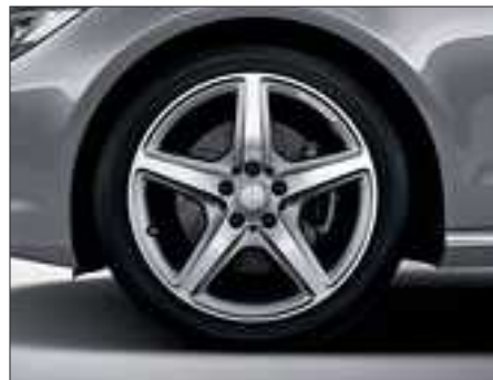
5-spoke AMG light-alloy wheels with 255/40 R 18 front and 285/35 R 18 rear tyres, painted in titanium grey with a high-sheen finish (standard for AMG Sports package, Code 790).
